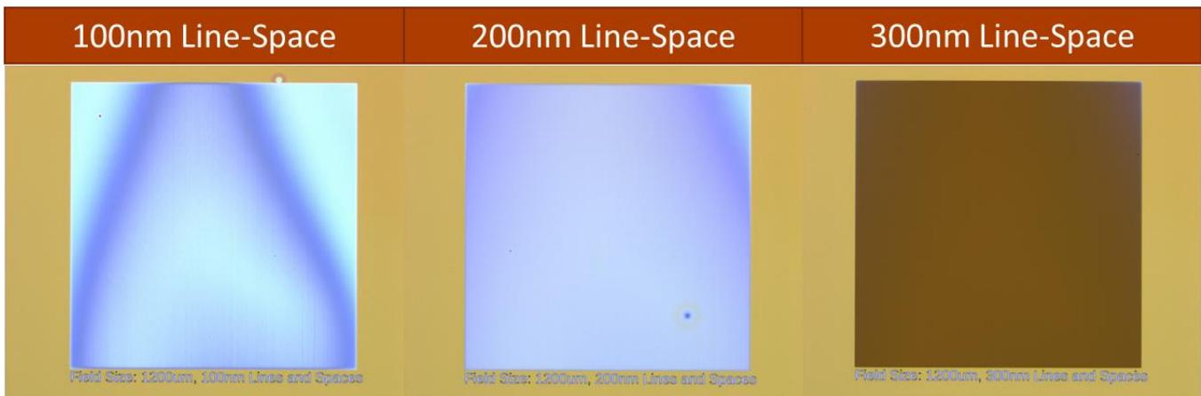
In the final image, field uniformity for 80 lines on a 160 nm pitch can be seen optically. One can deduce that the largest recommended field size to print critical features  $\geq 80\text{nm}$  is roughly  $150\ \mu\text{m}$  to maintain reasonable CD uniformity throughout the field.
