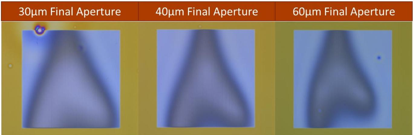
In the images below, using a 30um final aperture, distortion is apparent as a function of critical dimension. Reading from left to right, the line width increases. Optically, the image with the 300nm lines appears more uniform (except for some slight vignetting in the top left and right corners). As features scale down (reading right to left), the lack of dynamic focus in the tool becomes apparent.
