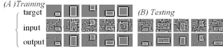
Figure 3: Square shape detection and enhancement. The Shape Graph weights W(Edge_{x_i, \theta_j}, Edge_{x_{i'}, \theta_{j'}}) = f(x_{i'} - x_i, \theta_{j'} - \theta_j) are learned with 50 training examples on image size = 100 \times 100 . f has a total of 4096 free parameters to be learned (edge position displacements \delta_x = \delta_y = 16 , edge orientation displacements \delta_\theta = 4 ).
