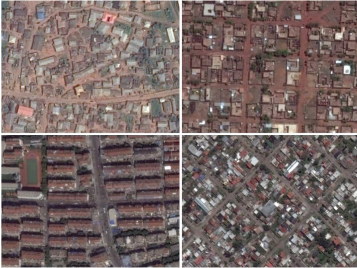
Figure 1: Four types of residential land use identified in the Atlas of Urban Expansion: Atomistic settlements (top left), informal subdivisions (top right), formal subdivisions (bottom right), and housing projects (bottom left). Source: Angel et al (2016).
