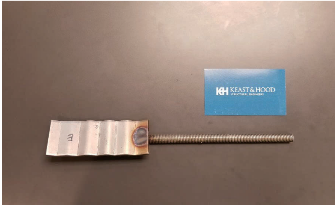
Figure 33. Anchor used to install cast-stone on College Hall, Keast & Hood Collection. (Photograph by author, 2019)
