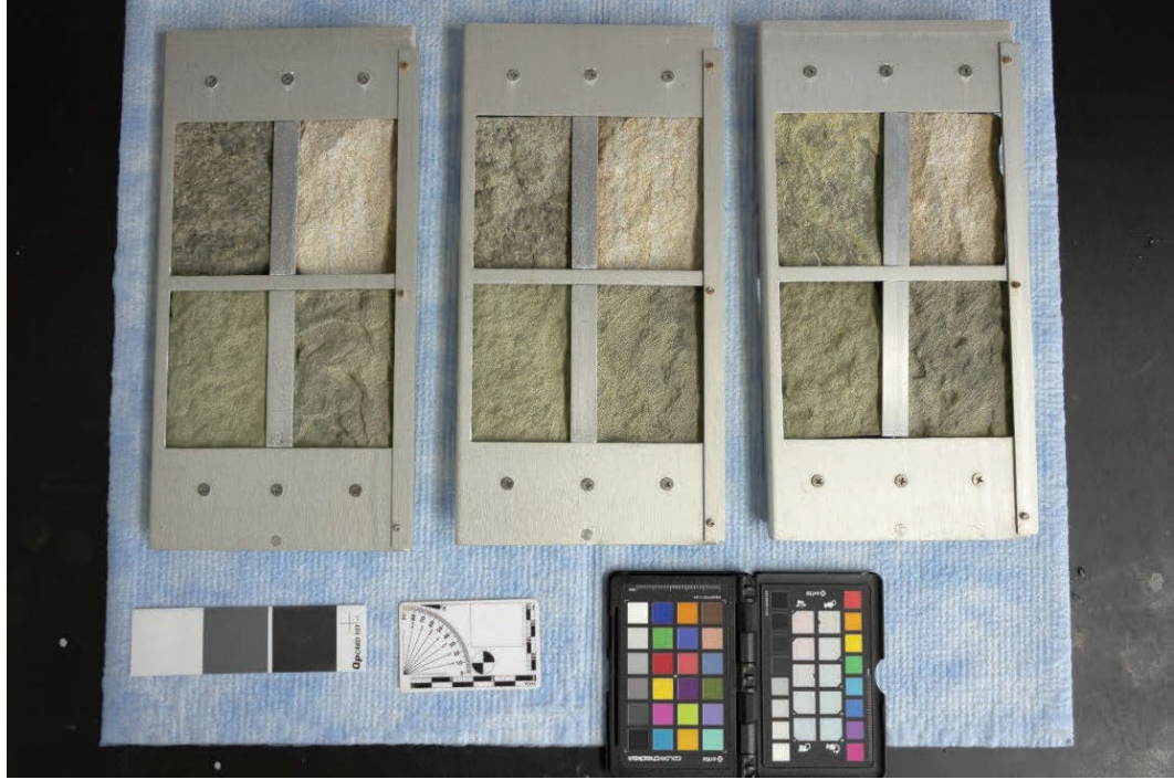
Figure 5. Testing surface, facing the UVB lamps and spray nozzles. (Photography by author, 2019)
