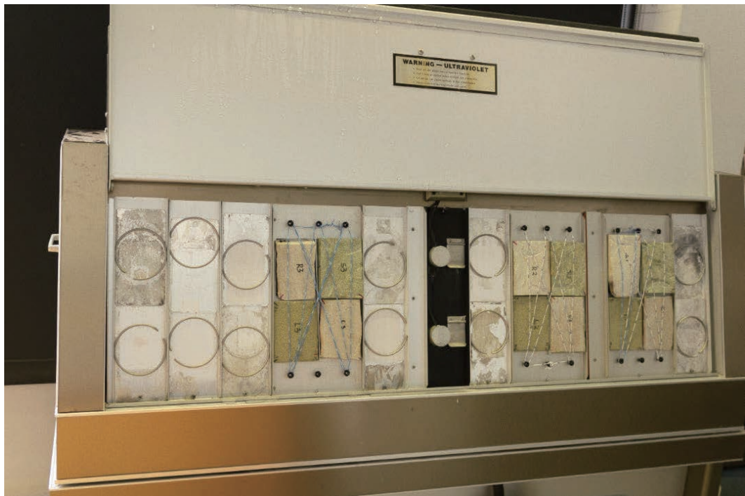
Figure 6. Samples placed in the weatherometer. (Photography by author, 2019)
