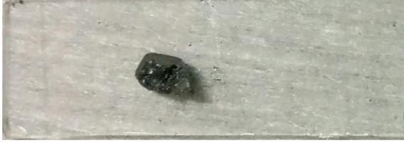
Figure 2.6: A crystal of the perovskite methylammonium lead iodide attached to a glass substrate using double-sided Scotch tape. The width of the substrate is 25.2 mm.
