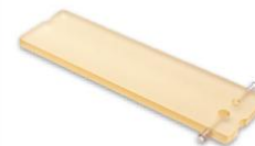
Figure 3C. A diverter plate for bench-scale single-pass TFF setup.
