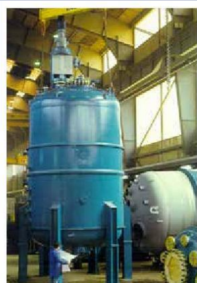
Stripper 60m 3 Eccentric agitation
