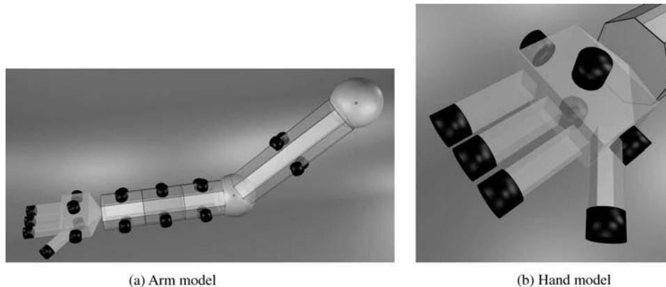
**Figure 2.** Arm and hand models with tactor placements.
