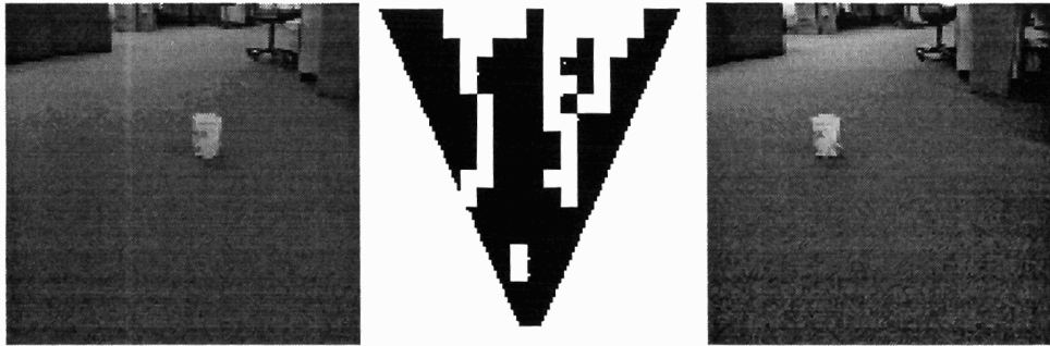
Figure 7: a) Left Image; b) Map of the free space in lower resolution (obstacles in white); c) Right Image
