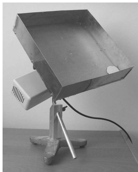
FIG. 2. The wearing apparatus used for the laboratory experiments. The rotating metal tray is  $30 \times 30 \times 7$  cm<sup>3</sup>.
