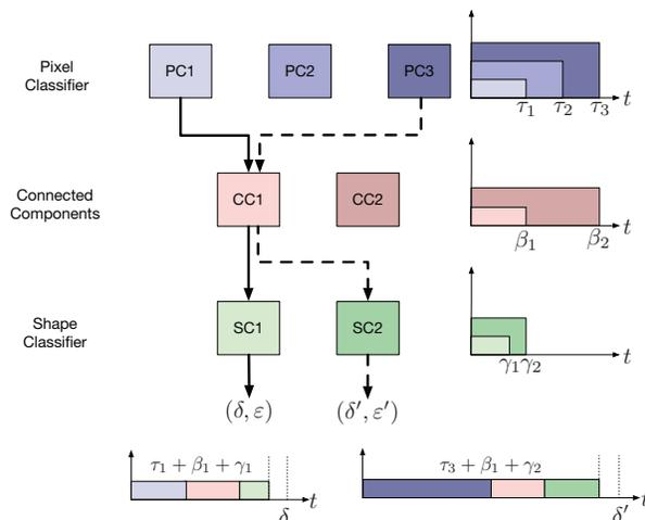
Fig. 6. Illustration of the various components used to compose the contract based perception algorithm and their representation as real-time tasks. For a given  $(\delta, \epsilon)$  contract, knob settings are chosen at run-time resulting in a schedule to execute these sequential components, or tasks, to respect the contract.
