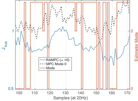
Fig. 10. Tracking cost at each time step for MPC (fixed mode 0 estimator) and RAMPC with  $\alpha = 0$ . Note how the RAMPC performs better (lower cost) than the MPC and there is dynamic switching of estimator modes at runtime leading to improved performance for the RAMPC.
