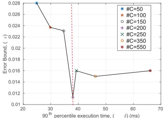
Fig. 8. Error-delay curve for the SVO algorithm running on the Odroid-U3 with different settings of maximum number of features ( $\#C$ ) to detect and track. The vertical line shows the cut-off for maximum delay and the SVO settings that are allowable for closed loop control of a hexrotor at 20Hz.
