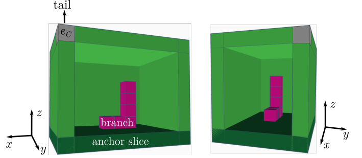
Fig. 7. An in-branch in a non-convex hole (two view angles with different sides transparent since the hole is closed in 3D). The dark green slice at the bottom is the anchor slice, the middle pink modules are the in-branch. Since e_{\mathcal{C}} (the (+z, +y, +x) extreme) is in the top slice, the bottom slice is the only slice which can be selected as next for deconstruction.
