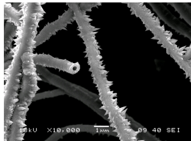
Fig. 7. A palladium cylinder is shown where the hollow interior is exposed. Notice the asymmetry in the wall thickness in sections of the cylinder as result of the line-of-sight deposition. The mean fiber diameter, previous to the Pd deposition, was 250 nm.
