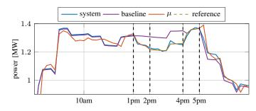
Fig. 6: The reference power signal is closely tracked by GP model providing sustained curtailment of 90 kW (with respect to the baseline) during the Demand Response event 2-4pm. Due to 1hr horizon in the control problem, the curtailment starts at 1:15pm, and the controller is further active until 5pm to reduce kickback.
