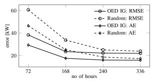
Fig. 3: Error in prediction of power consumption on test dataset. RMSE denotes root mean square error and AE denotes absolute error. The errors are much lower with optimal experiment design based on information gain. The random sampling requires  $2 \times$  time to reach the same accuracy as OED.
