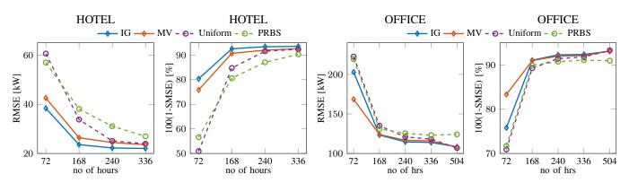
Fig. 5: Comparison of model accuracies for different experiments: OED based on information gain (IG), OED based on maximum variance (MV), uniform random sampling (Uniform) and pseudo random binary sampling (PRBS) for two buildings: hotel and office. RMSE denotes root mean square error and SMSE standardized mean square error; lower RMSE and higher 1-SMSE indicate better prediction accuracy.
