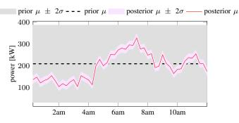
Fig. 2: Example of priors calculated using (1) and posteriors using (2) for predicting power consumption of a building for 12 hrs. Initially the mean is constant because  $\mu(x)$  is constant, and we observe a high variance. The posterior agrees with the actual power consumption with high confidence.
