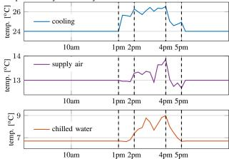
Fig. 8: Optimal set-points obtained after solving optimization (21).
