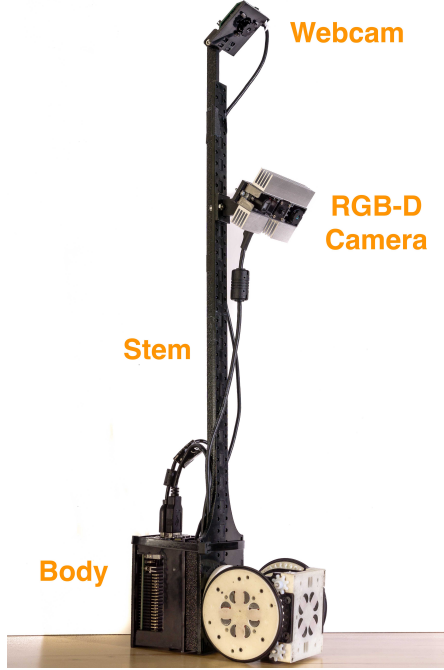
Figure 47: Sensor Module with labelled components. UP board and battery are inside the body.
