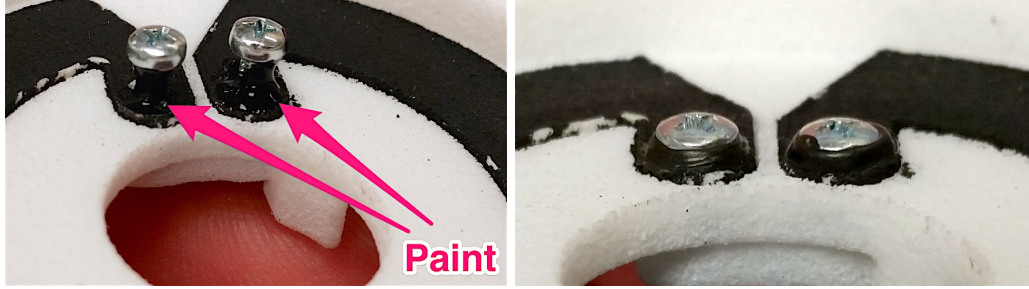
Figure 19: A bead of conductive paint applied beneath the screw head forms a good electrical connection with the track.
