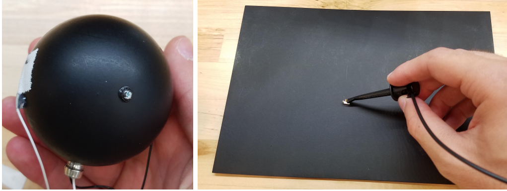
Figure 26: Left: Spherical PaintPot that senses position on the top hemisphere. Right: Flat-sheet PaintPot capable of sensing the X-Y position of the wiper.
