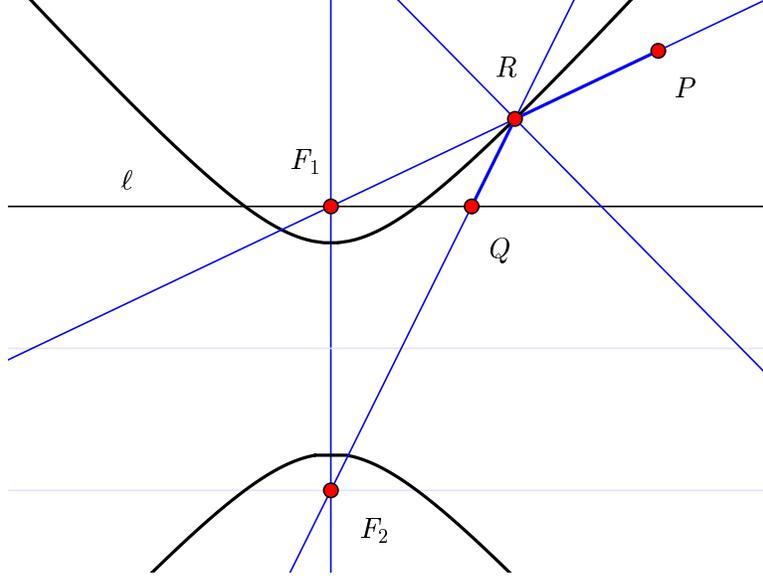
Figure 4: In general a conic reflects any ray of light incident with one of its foci (here  $F_1$ ) to a ray of light incident with its other focus ( $F_2$ ). Central catadioptric devices utilize this property and achieve a single effective viewpoint at one of the foci of a conic ( $F_1$ ).
