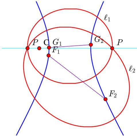
Figure 8: The two ellipses  $\ell_1$  and  $\ell_2$  are projections of two lines in space containing the point  $P$ . Their foci  $F_1, F_2$ , and  $G_1, G_2$  respectively lie on a hyperbola containing the foci of *all* ellipses through  $P$ . The foci of this hyperbola are the points in  $P$ . The point  $C$  is the image center.
