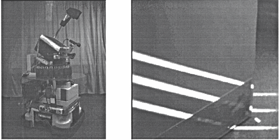
Figure C.1: Left: The mobile robot with the line striper. The line striper is the thing on the top that resembles an overhead projector. This is not a coincidence. Right: A typical image recorded by the line striper CCD camera showing the light stripes projected onto a partly opened door. Normally, the aperture of the camera would be smaller, so that only the light stripes would be visible in the image.
