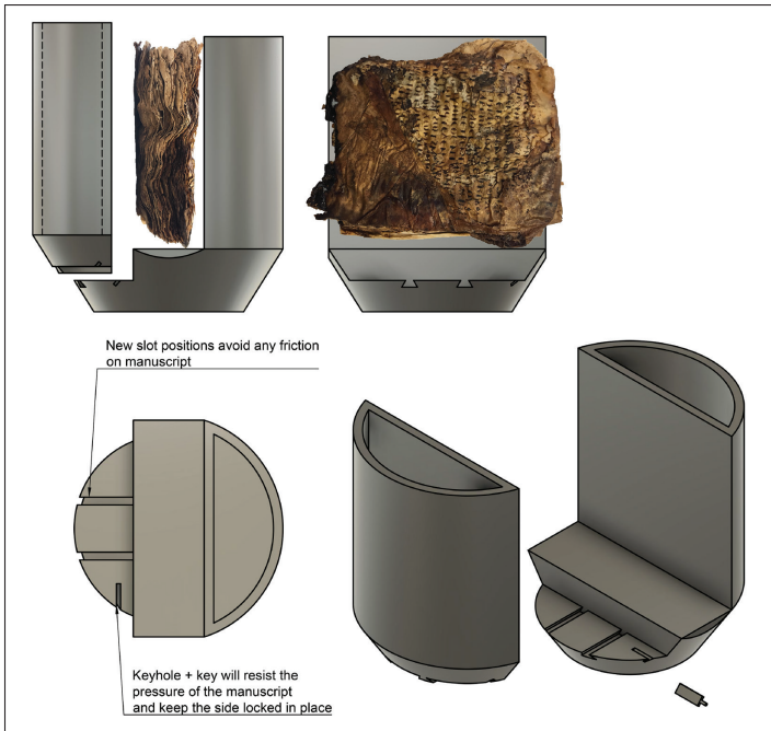
FIGURE 1. Illustration of the cylindrical shape of the mount and its assembly process.
