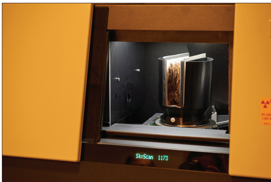
FIGURE 3. The manuscript encased, binding down, in the micro-CT machine. The black circular base remained in the scanner, allowing the manuscript case to be easily, gently, and securely installed using nylon set screws.
