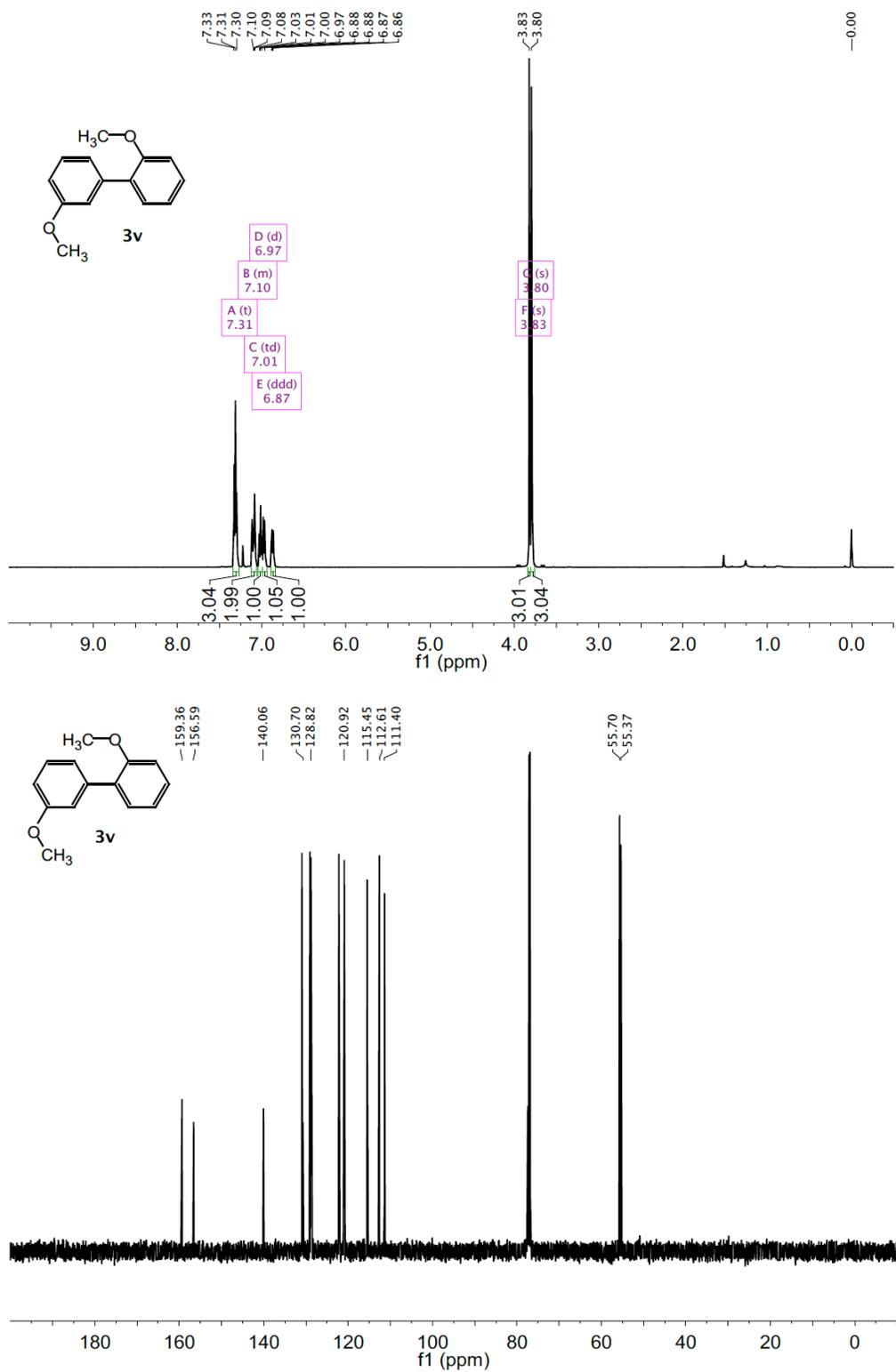
**Figure SF 4.22.**  $^1\text{H}$  NMR (top, 500 MHz) and  $^{13}\text{C}$  NMR (bottom, 125 MHz) spectra of 2,3'-dimethoxy-1,1'-biphenyl (**3v**) in  $\text{CDCl}_3$
