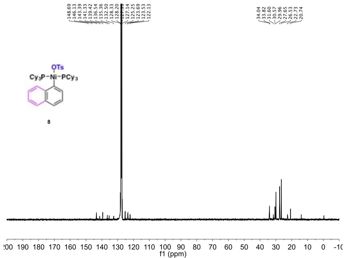
**Figure SI 26.**  $^1\text{H}$  NMR (top, 500 MHz),  $^{31}\text{P}$  NMR (middle, 203 MHz) and  $^{13}\text{C}$  NMR (bottom, 125 MHz) spectra of  $\text{Ni}^{\text{II}}\text{OTs}(1\text{-naphthyl})(\text{PCy}_3)_2$  in  $\text{C}_6\text{D}_6$ .
