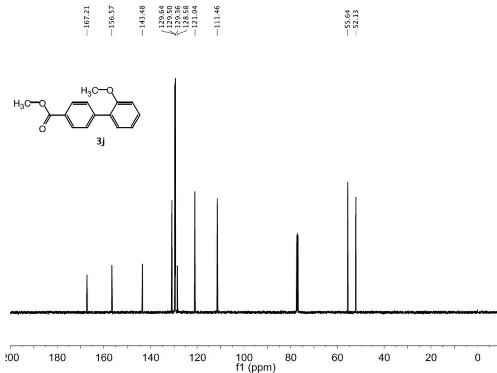
**Figure SF 4.10.** <sup>1</sup>H NMR (top, 500 MHz) and <sup>13</sup>C NMR (bottom, 125 MHz) spectra of methyl 2'-methoxy-[1,1'-biphenyl]-4-carboxylate (**3j**) in CDCl<sub>3</sub>.
