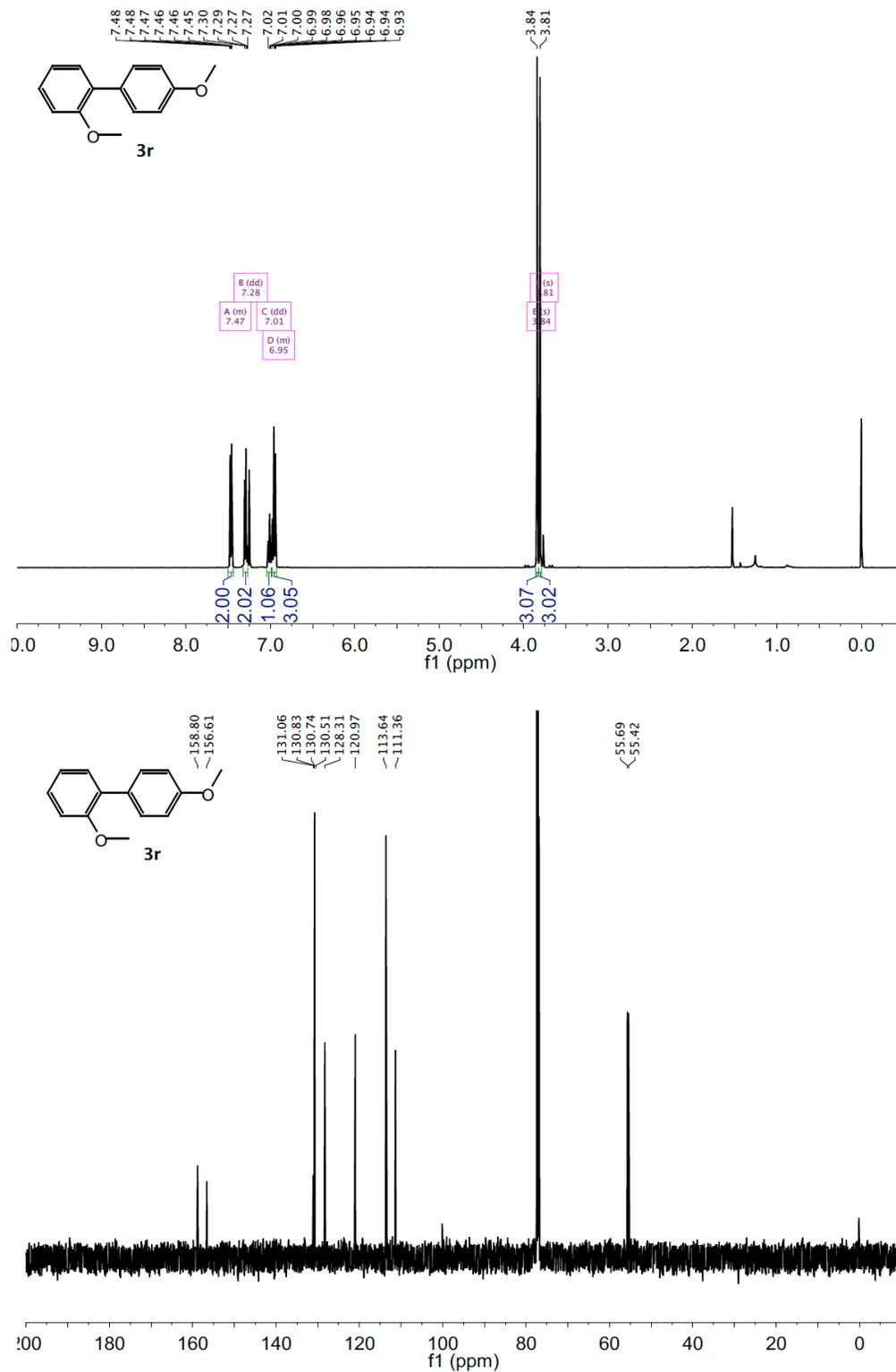
**Figure SF 4.18.** <sup>1</sup>H NMR (top, 500 MHz) and <sup>13</sup>C NMR (bottom, 125 MHz) spectra of 2,4'-dimethoxy-1,1'-biphenyl (**3r**) in CDCl<sub>3</sub>
