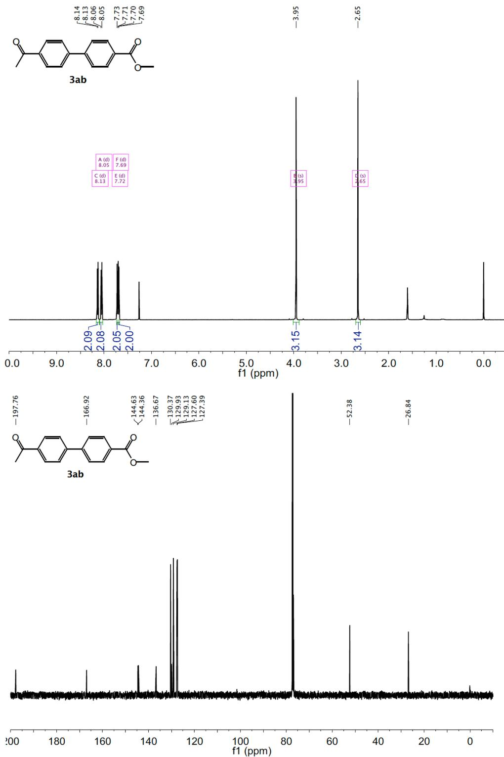
**Figure SF 4.28.** <sup>1</sup>H NMR (top, 500 MHz) and <sup>13</sup>C NMR (bottom, 125 MHz) spectra of methyl 4'-acetyl-[1,1'-biphenyl]-4-carboxylate (**3ab**) in CDCl<sub>3</sub>
