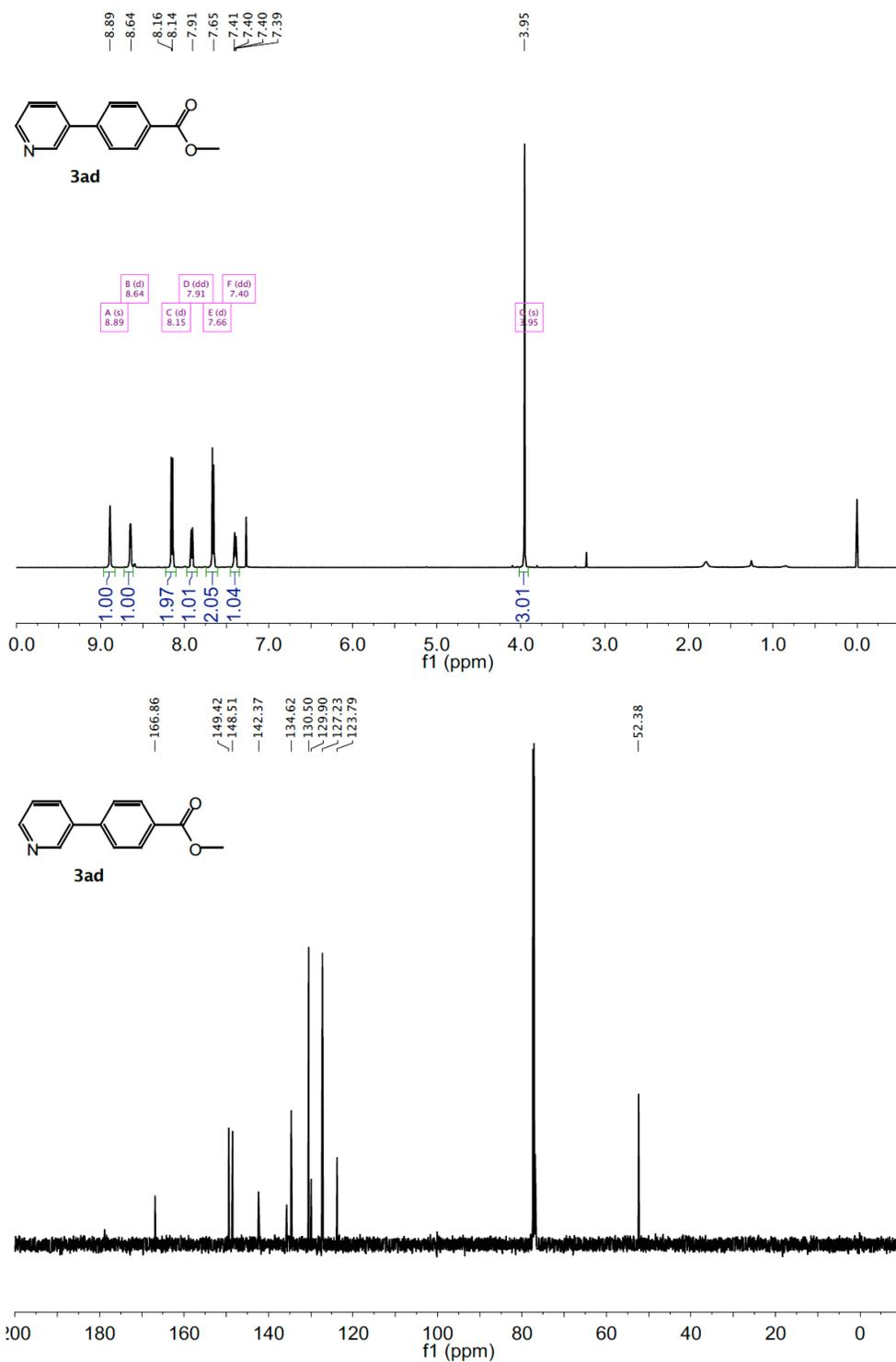
**Figure SF 4.30.** <sup>1</sup>H NMR (top, 500 MHz) and <sup>13</sup>C NMR (bottom, 125 MHz) spectra of methyl 4-(pyridin-3-yl)benzoate (**3ad**) in CDCl<sub>3</sub>
