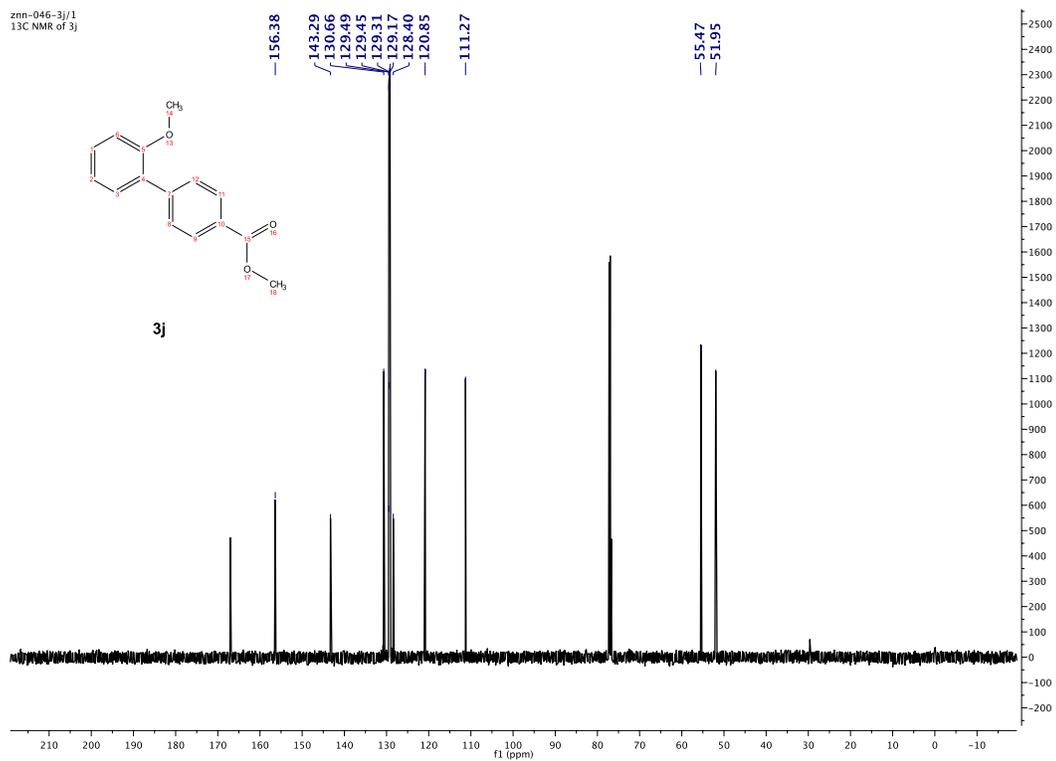
Figure SI 17. <sup>1</sup>H NMR (top, 500 MHz), and <sup>13</sup>C NMR (bottom, 125 MHz) spectra of **3j** in CDCl<sub>3</sub>.
