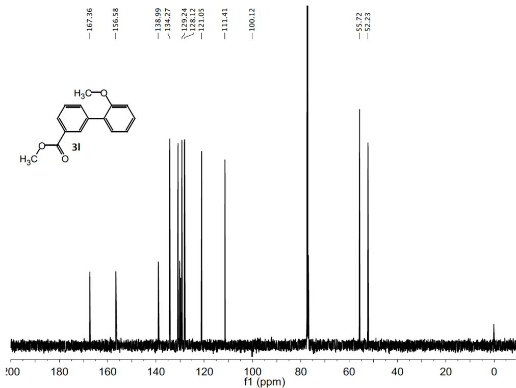
**Figure SF 4.12.** <sup>1</sup>H NMR (top, 500 MHz) and <sup>13</sup>C NMR (bottom, 125 MHz) spectra of methyl 2'-methoxy-[1,1'-biphenyl]-3-carboxylate (**3I**) in CDCl<sub>3</sub>.
