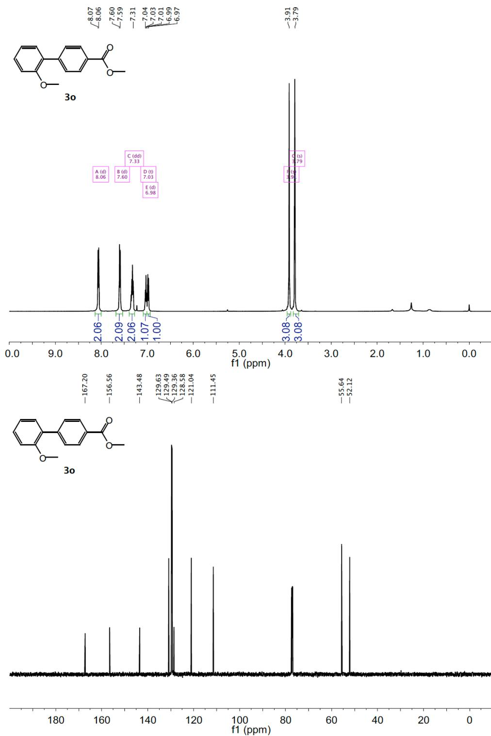
**Figure SF 4.15.** <sup>1</sup>H NMR (top, 500 MHz) and <sup>13</sup>C NMR (bottom, 125 MHz) spectra of methyl 2'-methoxy-[1,1'-biphenyl]-4-carboxylate (**3o**) in CDCl<sub>3</sub>.
