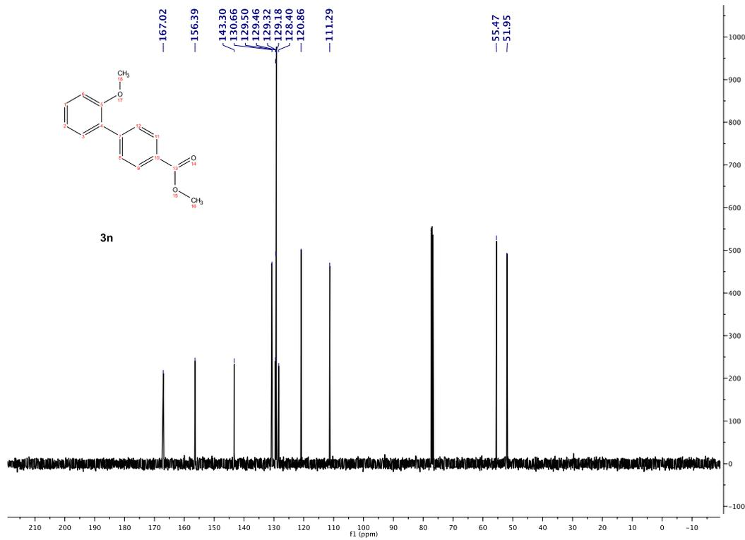
Figure SI 21. <sup>1</sup>H NMR (top, 500 MHz), and <sup>13</sup>C NMR (bottom, 125 MHz) spectra of **3n** in CDCl<sub>3</sub>.
