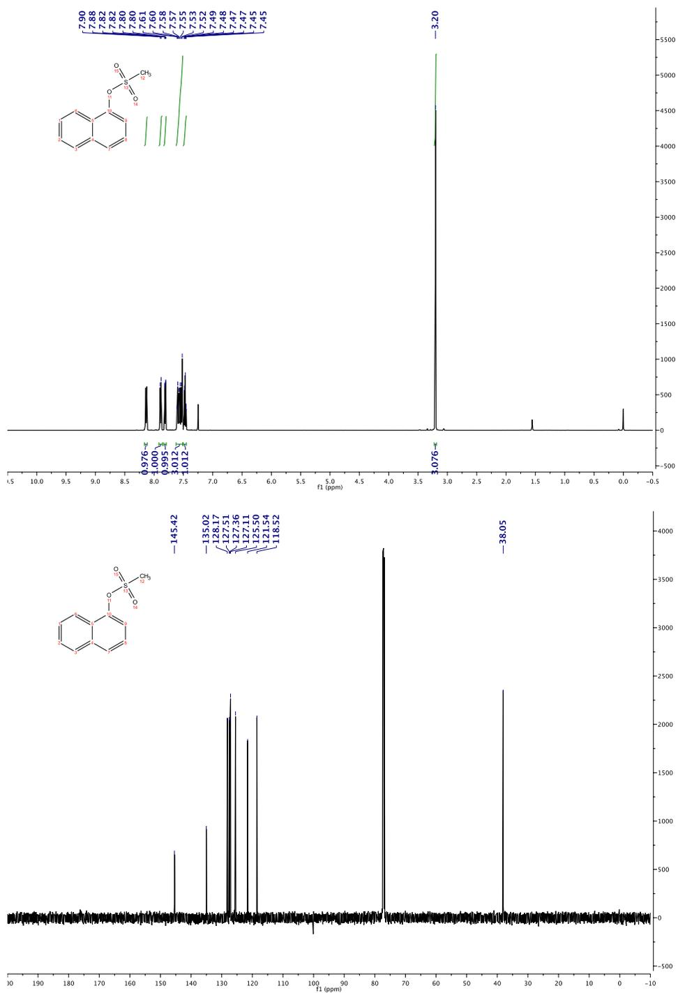
**Figure S1 2.**  $^1\text{H}$  NMR (top, 500 MHz), and  $^{13}\text{C}$  NMR (bottom, 125 MHz) spectra of 1-naphthyl methanesulfonate in  $\text{CDCl}_3$ .
