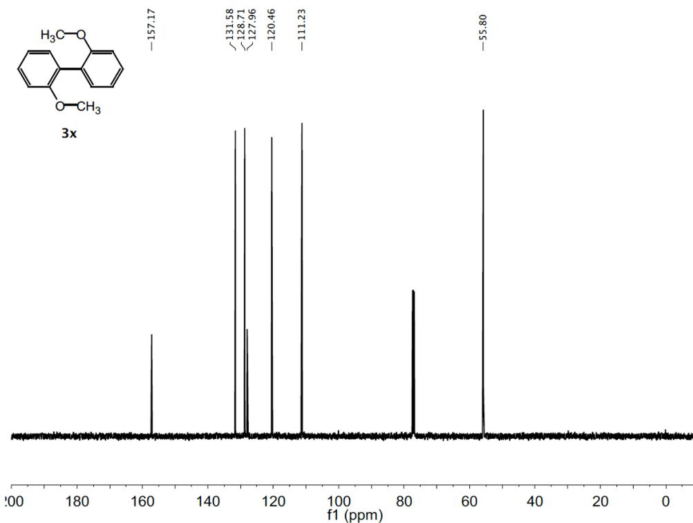
**Figure SF 4.24.** <sup>1</sup>H NMR (top, 500 MHz) and <sup>13</sup>C NMR (bottom, 125 MHz) spectra of 2,2'-dimethoxy-1,1'-biphenyl (**3x**) in CDCl<sub>3</sub>
