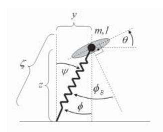
Fig. 1. Coordinate convention of SLIP with pitching dynamics. In the text, the COM coordinates are parametrized by Cartesian coordinates, i.e.,  $y = \zeta \sin(\psi)$  and  $z = \zeta \cos(\psi)$ . In flight, the leg angle  $\phi$  is in general a function of time and of the SLIP's liftoff state:  $\phi(t, x_0)$ .
