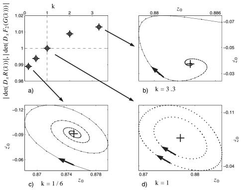
Fig. 3. (a) Comparison of the numerically computed determinant  $|\det(D_x R(\bar{x}))|$  (+) of the return map Jacobian to the determinant  $|\det(D_x F_2(G(\bar{x})))|$  (o) obtained by using the numerically determined fixed points in eq. (50). (b)–(d) Trajectories around a fixed point. Because of slow convergence, only every ninth iteration in plot (b) and every fifth iteration in plot (c) are shown.
