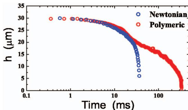
FIG. 3. (Color) Filament thickness  $h$  as a function of time for both Newtonian and polymeric fluids at the same flow rates.
