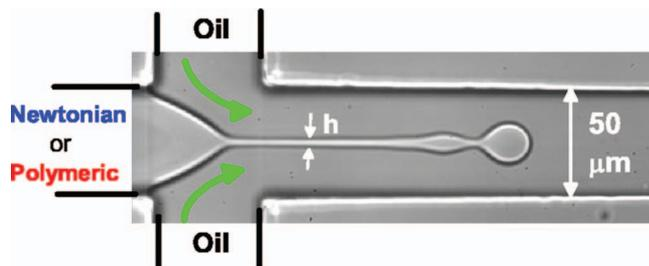
FIG. 1. (Color) Microchannel experimental setup. The device is  $50\ \mu\text{m}$  wide and  $30\ \mu\text{m}$  deep. Oil is used as the continuous phase. Newtonian or polymeric fluids are used as dispersed phases.
