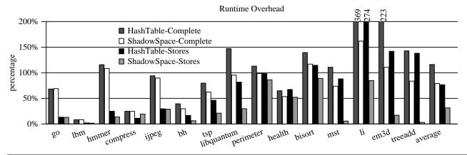
Figure 2. Normalized execution time overhead of SoftBound with full checking and store-only checking with two metadata organizations.
