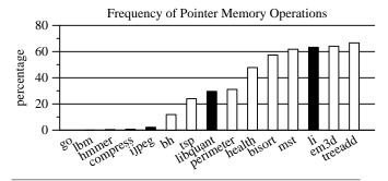
**Figure 1.** Percentage of the memory operations that load or store a pointer from/to memory, thus requiring a metadata access. The SPEC benchmarks are shaded dark.
