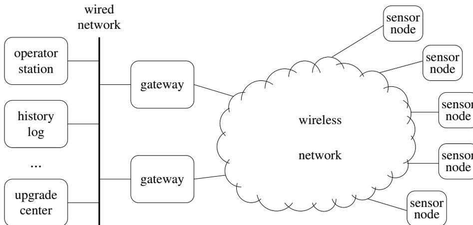
Figure 6: System architecture for the case study
