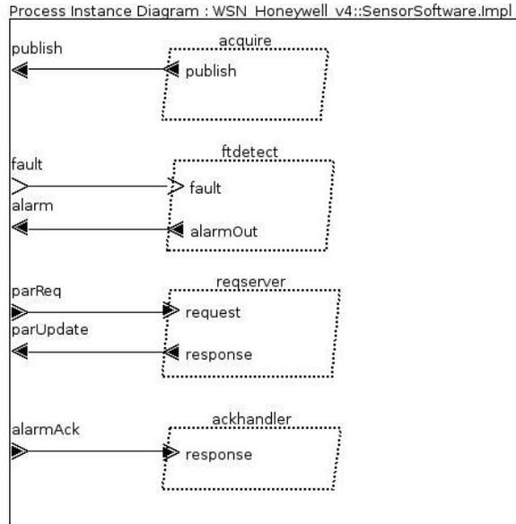
Figure 9: AADL architecture of the sensor node
