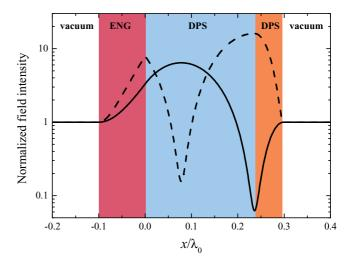
FIG. 2. (Color online) Resonant electric (solid) and magnetic (dashed) field intensity distributions (normalized by the incident fields) for a configuration as in Fig. 1, with  $\varepsilon_1 = -3$ ,  $d_1 = 0.1\lambda_0$ ,  $\varepsilon_2 = 2.5$ ,  $d_2 = 0.236\lambda_0$ ,  $\varepsilon_3 = 16$ , and  $d_3 = 0.0624\lambda_0$ .
