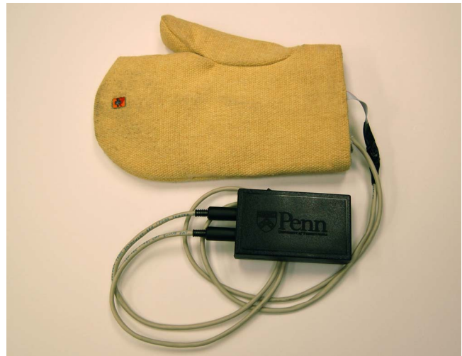
Figure 2: The SlipGlove V1. A single slip sensor has been placed in the area of the wearer's middle finger. The off-glove control box is wired to the glove via flexible cabling, and it can be clipped comfortably on the user's belt. This glove was used for all experiments described in this paper.
