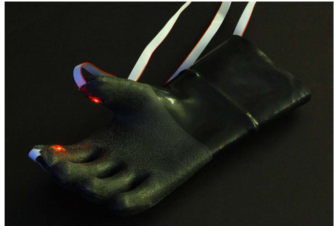
Figure 1: The SlipGlove V2. Note the presence of relative motion sensors on the inside of the thumb and index finger, with wires leading to an off-glove control box. When objects slide over the sensors, actuators inside the glove vibrate in response to the slip information.
