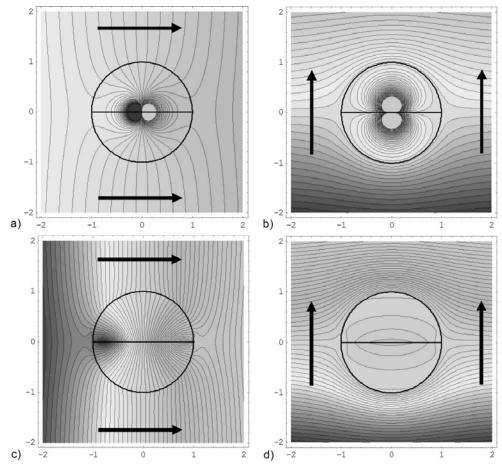
Figure 1 – Potential distribution around and inside the 3-D plasmonic spherical nanoswitch at resonance in the ideal case ( $\varepsilon_1 = -\varepsilon_2 = 16\varepsilon_0$ ) for parallel (panel a) and series configuration (panel b); introducing realistic losses and permittivity mismatch  $\varepsilon_2 = (-16.1 - j\,0.2)\varepsilon_0$  in the spherical particles for parallel (panel c) and series (d) configurations. Darker regions correspond to larger values.
