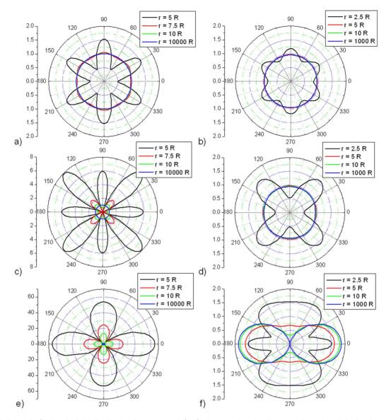
FIG. 2. (Color online) Electric-field distribution in the  $\theta = \pi/2$  (x-y) plane varying the distance r from the origin for the resonant loop of Fig. 1 with (a)  $R = \lambda_b/100$ , N = 6, (b)  $R = \lambda_b/10$ , N = 6, (c)  $R = \lambda_b/100$ , N = 4, (d)  $R = \lambda_b/10$ , N = 4, (e)  $R = \lambda_b/100$ , N = 2, and (f)  $R = \lambda_b/10$ , N = 2.
