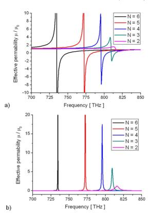
FIG. 3. (Color online) (a) Real and (b) imaginary parts of the effective permeability for a cubic lattice with number density  $N_d$  =  $(160 \text{ nm})^{-3}$  made of nanoloops with radius R=60 nm each of which is composed of N silver particles with radius a=24 nm.
