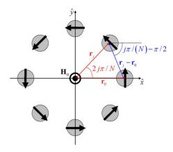
FIG. 1. (Color online) A nanoring made of *N* nanoparticles symmetrically displaced around the origin of a Cartesian reference system in the *x-y* plane. The electric polarization response to a uniform magnetic excitation is depicted in the figure, ensuring purely rotational induced electric dipoles (black arrows).
