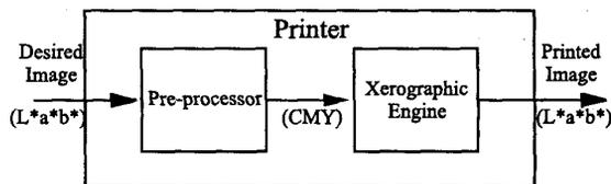
**Figure 1:** Decomposition of a xerographic printer into the print engine and pre-processor. The engine embodies the transformation  $T$ , while the pre-processor performs an approximation of the inverse  $\tilde{T}^{-1}$ , such that  $T \circ \tilde{T}^{-1}$  is approximately the identity for within gamut colors.
