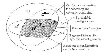
Figure 2: Constraining the configurations space to ensure safety
