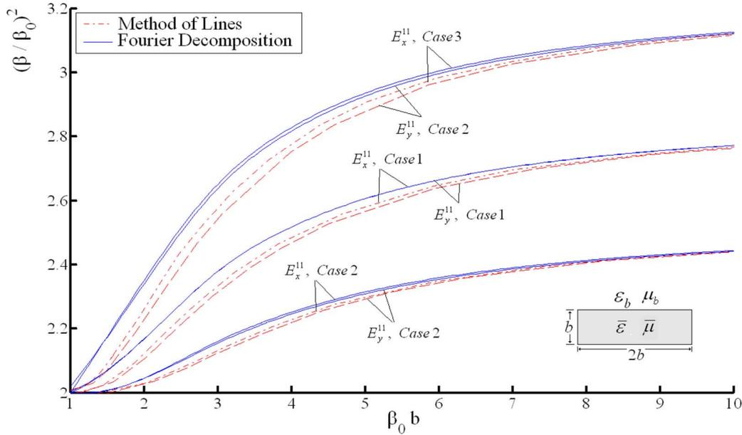
Fig. 6. Dispersion curves of illustrated channel waveguide with permittivity and permeability tensors.  $\alpha_x = 2.5b$ ,  $\alpha_y = b/2$ , and  $\rho = \sqrt{\alpha_x \alpha_y}$ . Field expansions include 15 terms in each direction.
