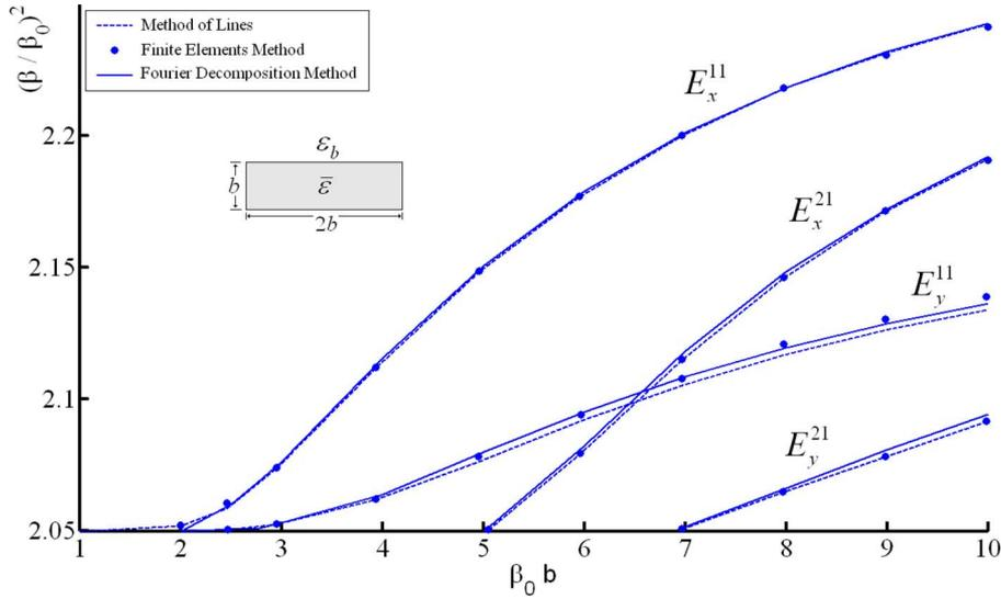
Fig. 2. Dispersion curves for the first four modes of the illustrated channel waveguide. Relative permeability tensor of the channel is  $\epsilon_x = \epsilon_z = 2.31$ ,  $\epsilon_y = 2.19$ , and  $\epsilon_b = 2.05$  for background.  $\alpha_x = b$ ,  $\alpha_y = b/2$ , and  $\rho = \sqrt{\alpha_x \alpha_y}$ . Expansions with 15 terms in each direction are used.
