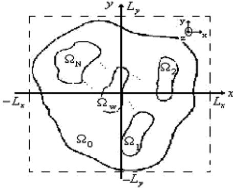
Fig. 1. Dielectric waveguiding structure with arbitrary shaped anisotropic inhomogeneous dielectric subregions  $\Omega^1, \Omega^2, \Omega^3, \dots, \Omega^N$  and  $\Omega^w$  embedded in  $\Omega^0$  dielectric media.
