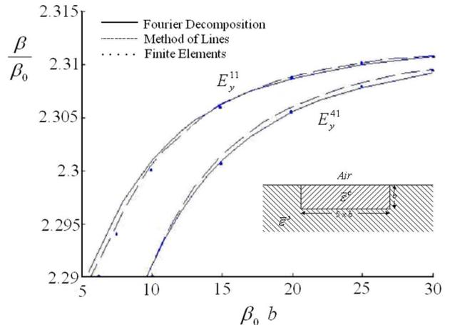
Fig. 4. Dispersion curves for the  $E_y^{11}$  and  $E_y^{41}$  modes of the illustrated waveguide. Relative permeability tensor in the channel is  $\epsilon_x^c = 2.22^2$ ,  $\epsilon_y^c = \epsilon_z^c = 2.3129^2$ , and in the substrate,  $\epsilon_y^s = \epsilon_z^s = 2.29^2$ , for background. In this case,  $b = 1.0 \mu\text{m}$ ,  $\alpha_x = 2.5b$ ,  $\alpha_y = b/2$ , and  $\rho = \sqrt{\alpha_x \alpha_y}$ . Field expansions with 15 terms in each direction.
