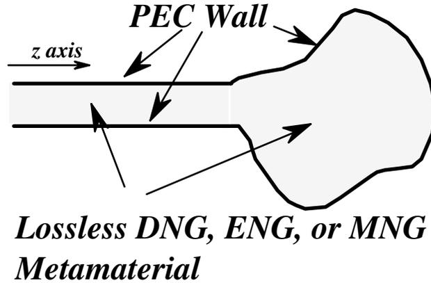
Fig. 1. Geometry of the problem. A one-port termination filled with an isotropic lossless double-negative (DNG) ( $\epsilon < 0, \mu < 0$ ), epsilon-negative (ENG) ( $\epsilon < 0, \mu > 0$ ), or mu-negative (MNG) ( $\epsilon > 0, \mu < 0$ ) metamaterial.
