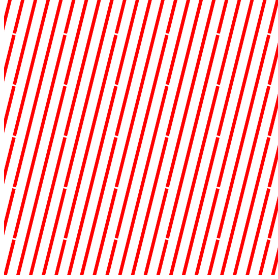
Figure 1: An example gangbuster surface. In this illustration, the radius of the dipoles is exaggerated five times in order to be visible in print. The parameters D = 0.13\Lambda , L = 0.533\Lambda , a = 0.001\Lambda , and n = 4 were used to construct this surface (see text and Figure 2 for parameter explanations). From these parameters, one can compute \alpha = 14.0^\circ , d_{\text{near}} = 0.0315\Lambda , and d_{\text{end}} = 0.006\Lambda . Here \Lambda is some reference length that may be chosen to scale this surface to any desired physical dimension.
