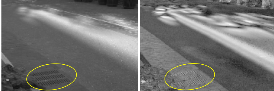
Fig. 3. Images in Fig. 2 are contrast-enhanced by linear intensity range stretch followed by gamma correction of 0.5 to show the details in the dark area. Left: intensity image. Right: degree of polarization image. It is clear that the pattern revealed in the polarization image is not present in the intensity image even after contrast enhancement. The yellow circle points out the same sewage drain cover that is visible in all related pictures up to Fig. 4 except Fig. 4 Left to help orientation.
