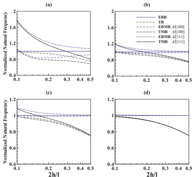
FIG. 3. (Color online) Effect of beam thickness on the nondimensional fundamental natural frequency of the microbeams for  $k=5/6$ , and different beam length: (a)  $l=10$  nm, (b)  $l=50$  nm, (b)  $l=100$  nm, and (d)  $l=1$   $\mu\text{m}$ .
