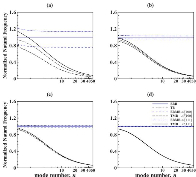
FIG. 4. (Color online) Effect of mode number on the nondimensional natural frequencies of the microbeams for  $2h=0.2l$ ,  $k=5/6$  and different beam length: (a)  $l=10$  nm, (b)  $l=50$  nm, (b)  $l=100$  nm, and (d)  $l=1$   $\mu\text{m}$ .
