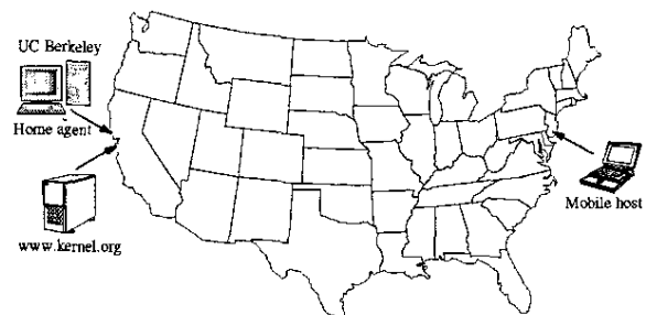
Fig. 11. The autonomous HA placement decision made by DHARMA. Notice how this allows the MH almost unrestricted movement without incurring additional routing overheads.
