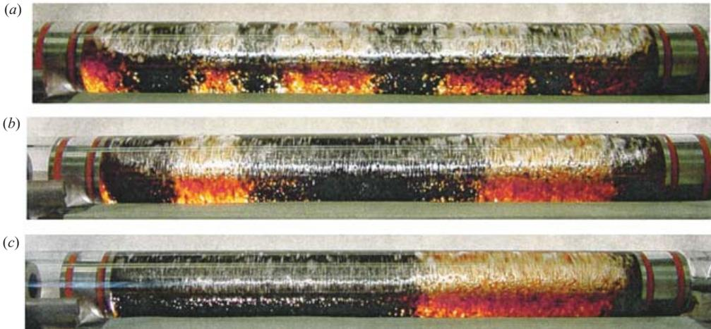
FIGURE 22. Segregation of two types of particle in a 47.8% aqueous glycerine solution with  $\rho_l = 1.09 \text{ g cm}^{-3}$ . The filling level  $F = 0.354$ . The concentrations of the black silicon particles and brown resin particles are 21.7% and 12%, respectively. The rotational speed is 165 r.p.m. (a) 30 min, (b) 2 h, (c) 20 h after the beginning of rotation.
