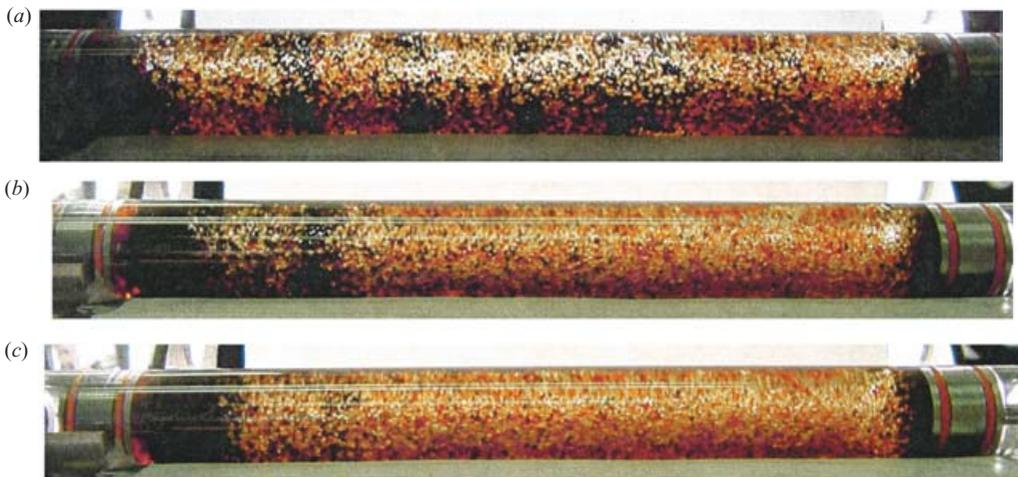
FIGURE 23. Segregation of two types of particle in a 48.7% aqueous glycerine solution. The filling level  $F = 0.328$ . The concentrations of the black silicon particles and brown resin particles are both 16%. The rotational speed is 160 r.p.m. (a) 4 min, (b) 24 min, (c) 36 min after the beginning of rotation.
