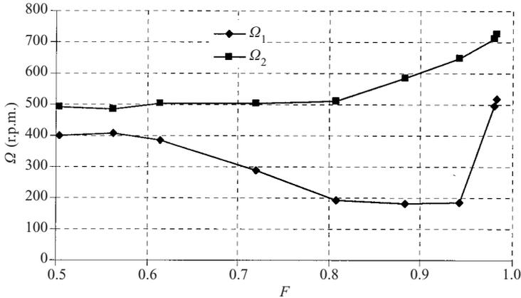
FIGURE 18. Critical conditions for the formation of bubbles in soybean oil. The experiments were carried out in a glass cylinder with an inner diameter of 1.28 cm and a length of 22.14 cm. When  $F < 0.4$ , a single air bubble is stable at any rotational speed. For  $F \geq 0.5$ , when the rotational speed is between  $\Omega_1$  and  $\Omega_2$ , separated bubbles are observed.
