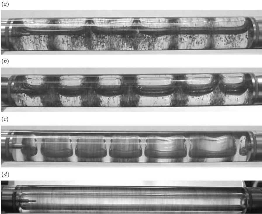
FIGURE 20. Particle segregation of resin particles with  $\rho_p = 1.13 \text{ g cm}^{-3}$  in the soybean oil with  $\rho_l = 0.915 \text{ g cm}^{-3}$ . The particle concentration is 15% and the filling level  $F = 0.6$ . (a)  $\Omega = 200 \text{ r.p.m.}$  (b)  $300 \text{ r.p.m.}$  (c)  $600 \text{ r.p.m.}$  (d)  $1000 \text{ r.p.m.}$
