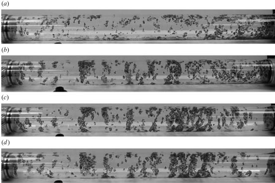
FIGURE 13. Band formation of particles due to capillarity. The liquid is water ( $18^{\circ}\text{C}$ ) and the particles are polymer particles. The filling level  $F$  is 0.041 and the particle concentration is 20.7%. The rotational speed  $\Omega = 8.57$  r.p.m.,  $\beta = 15.94$ , average film thickness  $D_a = 0.288$  mm, minimum film thickness  $D_{min} = 0.0213$  mm,  $D_{min}/d_p = 0.033$ . (a) 3 min, (b) 1.5 h, (c) 6 h, (d) 18 h after the beginning of rotation.
