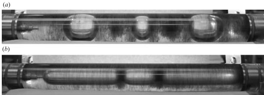
FIGURE 21. Particle segregation of resin particles with  $\rho_p = 1.13 \text{ g cm}^{-3}$  in glycerine with  $\rho_l = 1.173 \text{ g cm}^{-3}$ . The particle concentration is 8.96% and the filling level  $F = 0.667$ . (a)  $\Omega = 200 \text{ r.p.m.}$  (b)  $600 \text{ r.p.m.}$
