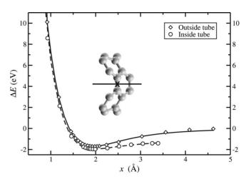
FIG. 5. Lithium interaction with nanotube vs distance to the wall. The Li is located on top of the center of a C-C bond. The diamonds represent the interaction from the outside and circles, the interaction from the inside. The lines represent fitted potentials (see text for details).
