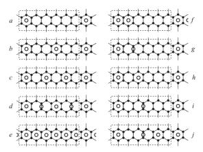
FIG. 6. A selection of configurations used to study Li-Li interactions inside the (5,5) tube. Only the carbon atoms (solid circles) close to the chain of Li atoms (empty circles) are shown for clarity. The solid lines represent C-C bonds and the dashed line shows the size of the 120 C supercell along the tube axis. The Li atoms are evenly spaced in the left column and unevenly spaced in the right column.
