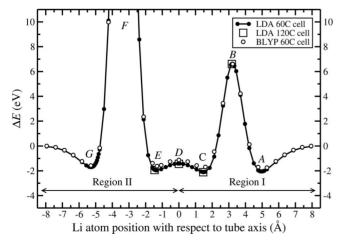
FIG. 3. The Li-tube interaction along a line perpendicular to the tube axis and passing though the center of a carbon hexagon (see Fig. 2). The labels are explained in the text and the corresponding energies are listed in Table II.
