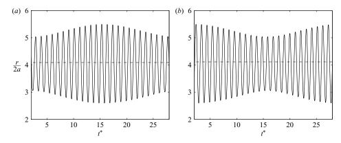
FIGURE 15. Radial positions of the particles as measured from the centre of their corresponding settling planes during the out-of-phase spiralling state. Here,  $Re_p \sim 5.6$  and  $Re_s \sim 1$ . Dotted lines indicate the fixed points on each settling plane about which the spiral orbital motions of the particles take place. (a) Particle 1; (b) particle 2.
