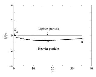
FIGURE 25. Axial migration of two particles with different densities but the same size released close to each other. The heavier of the two is released far away from its equilibrium point.
