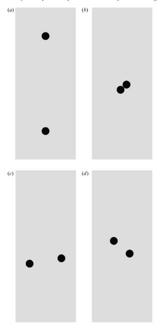
FIGURE 10. Snapshots of two-particle interaction dynamics at different times as viewed by an inertial observer in the  $(y_i, z_i)$ -plane. The cylindrical wall is not shown to scale here for clarity. (a) Initial position. (b) Kissing and tumbling at A. (c) Axial migration to B-B'. (d) Settling planes D-D'.
