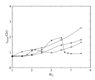
FIGURE 20. The axial positions of the settling planes of the particles as a function of  $Re_s$ .  $\Box$ ,  $\rho_p/\rho_f=0.98$ ,  $Re_p=5.6$ ;  $\triangle$ ,  $\rho_p/\rho_f=0.95$ ,  $Re_p=14.0$ ; \*,  $\rho_p/\rho_f=0.9$ ,  $Re_p=28.0$ ; \*,  $\rho_p/\rho_f=0.8$ ,  $Re_p=56$ .
