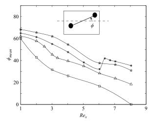
FIGURE 19. The angle  $\phi$  made by the line of centres of the two particles with the rotation (horizontal) axis (see inset) as a function  $Re_s$ .  $\Box$ ,  $\rho_p/\rho_f = 0.98$ ,  $Re_p = 5.6$ ;  $\triangle$ ,  $\rho_p/\rho_f = 0.95$ ,  $Re_p = 14.0$ ; \*,  $\rho_p/\rho_f = 0.9$ ,  $Re_p = 28.0$ ; \*,  $\rho_p/\rho_f = 0.8$ ,  $Re_p = 56$ .
