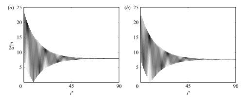
FIGURE 2. Comparison of radial position histories between (b) DNS and (a) the solution of (27) without the inclusion of lift and history forces. The parameters are:  $\rho_p/\rho_f = 0.8$ ,  $Re_p = 56$  and  $Re_s = 3$ . (a) Final fixed equilibrium point position is given by  $x_i/2a = -7.86$ ,  $y_i/2a = 0.85$ . (b) Final fixed equilibrium point position is given by  $x_i/2a = -7.7$ ,  $y_i/2a = 0.03$ .
