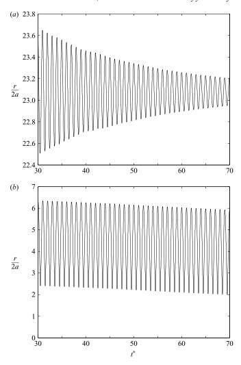
FIGURE 28. Normalized radial position histories of the particles released far away but closer to their respective equilibrium points. (a) Normalized radial position of the lighter of the two particles. (b) Normalized radial position of the heavier of the two particles.
