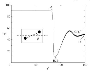
FIGURE 9. The angle  $\phi$  made by the line of centres with the horizontal axis (as shown in the inset schematic).  $\phi = 90^{\circ}$  implies the particles are in the same transverse planes and  $\phi = 0$  implies the lines of centres is aligned parallel to the axis of rotation. See figure 6 for the location of the points.
