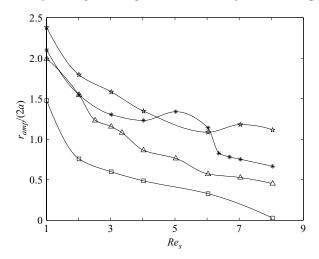
FIGURE 21. The amplitude of oscillation about the mean radial position of each individual particle as a function of  $Re_s$ . A value of zero implies an equilibrium fixed-point state.  $\Box$ ,  $\rho_p/\rho_f = 0.98$ ,  $Re_p = 5.6$ ;  $\triangle$ ,  $\rho_p/\rho_f = 0.95$ ,  $Re_p = 14.0$ ; \*,  $\rho_p/\rho_f = 0.9$ ,  $Re_p = 28.0$ ; \*,  $\rho_p/\rho_f = 0.8$ ,  $Re_p = 56$ .
