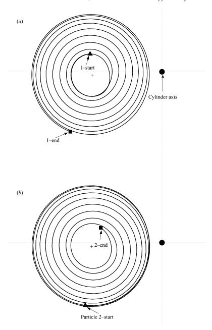
FIGURE 14. The trajectory as observed by an observer in an inertial frame on the transverse  $(x_i, y_i)$ -plane for  $Re_p \sim 5.6$  and  $Re_s \sim 1$  is shown for half the pedalling cycle (the period for which particle 1 spirals out while particle 2 spirals in).
