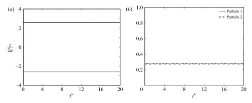
FIGURE 13. Numerical solutions of (b) radial position and (a) axial migration of two particles at stationary states for  $\rho_p/\rho_f = 0.98$ ,  $Re_p \sim 5.6$  and  $Re_s \sim 8$ .
