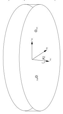
FIGURE 1. Schematic of the rotating wall vessel with 2 particles. z axis is the axis of rotation and the transverse plane is the x-y axis in a rotating frame. 1 and 2 denote the two spherical particles, respectively.
