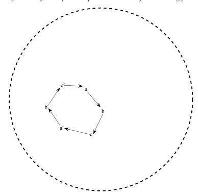
FIGURE 8. Discrete time snapshots of centres of the epitrochoidal trajectories of two-particles as viewed by an observer in a rotating frame (see figure 3). a–b–c and a'–b'–c' denote the discrete epitrochoidal centres of particles 1 and 2, respectively. This configuration of the leader–follower switches, as is evident from the figure. This process repeats until the interparticle gap is reduced and the particles start tumbling along the axial direction.
