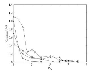
FIGURE 22. The amplitude of spiralling motion of each individual particle as a function of  $Re_s$ . A value of zero indicates a perfect circular pedaling motion.  $\Box$ ,  $\rho_p/\rho_f = 0.98$ ,  $Re_p = 5.6$ ;  $\triangle$ ,  $\rho_p/\rho_f = 0.95$ ,  $Re_p = 14.0$ ; \*,  $\rho_p/\rho_f = 0.9$ ,  $Re_p = 28.0$ ; \*,  $\rho_p/\rho_f = 0.8$ ,  $Re_p = 56$ .
