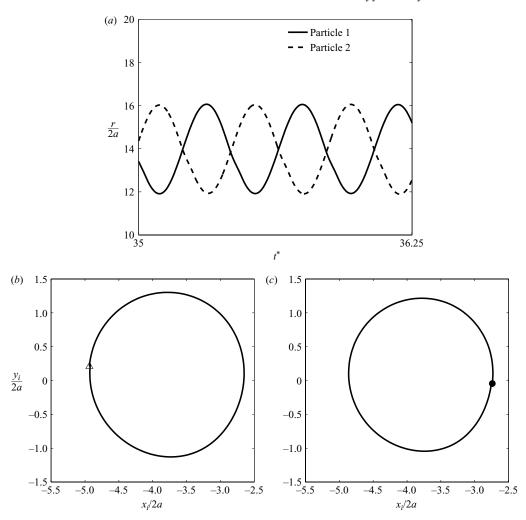
FIGURE 16. (a) Radial positions and (b,c) trajectories of particles as seen by an inertial observer corresponding to the case of  $\rho_p/\rho_f = 0.8$ ,  $Re_p \sim 60$  and  $Re_s \sim 6$ . The positions of particles  $1(\bullet)$  and  $2(\triangle)$  observed at the same instant showing the out-of-phase behaviour. The particles are seen to undergo near-circular bicycle pedalling motion.
