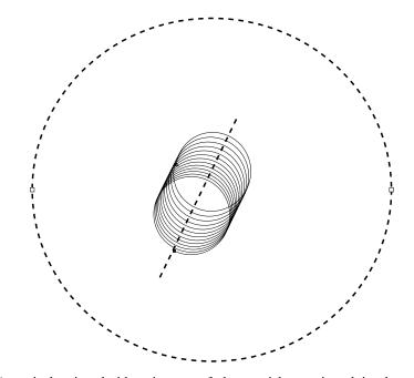
FIGURE 3. A typical epitrochoid trajectory of the particle as viewed in the rotating frame of reference for the case of single-particle dynamics. The dashed line circle represents the enclosing cylinder. The straight dashed line is the locus of the instantaneous centre of the epitrochoidal trajectory.
