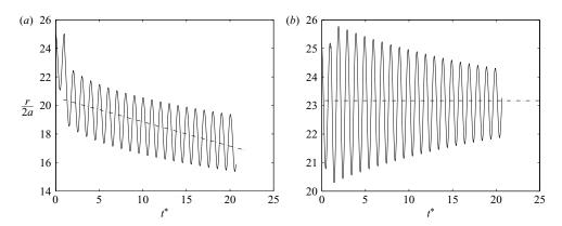
FIGURE 26. Normalized radial position histories of the particles released close to each other.
