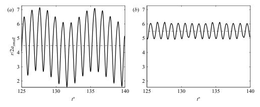
FIGURE 24. Radial positions of the particles as measured from the centres of their corresponding settling planes  $(x_i = y_i = 0)$  after the attainment of equilibrium states. (a) Smaller particle; (b) larger particle. Dotted lines indicate the fixed radial points on each settling plane about which the orbital motions of the particles take place. Here,  $a_{small}$  denotes the radius of the smaller particle.
