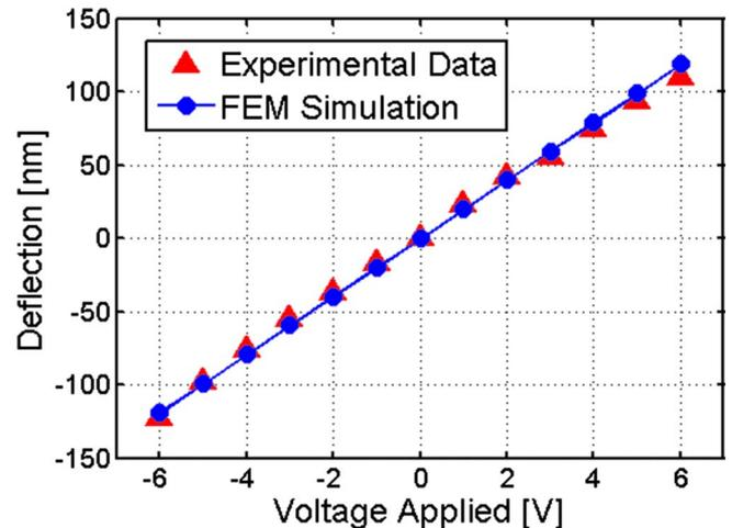
FIG. 2. (Color online) Excellent agreement exists between experimental data and FEM analysis of the vertical deflection for an 18  $\mu\text{m}$  long, 4  $\mu\text{m}$  wide, and 350 nm thick composite beam operated as a bimorph.
