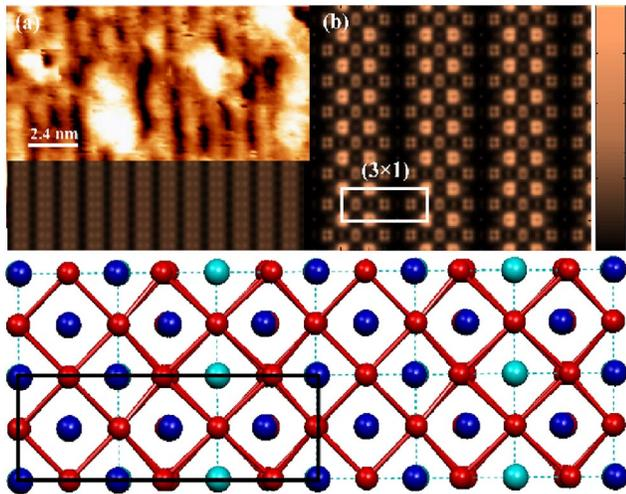
FIG. 3 (color online). (a) Comparison of STM and the computed LDOS of the predicted  $(3 \times 1)$  phase. (b) Atomic scale detail of the computed LDOS and (c) surface atomic structure for the same phase. Ba: cyan, Ti: blue, O: red. The color bar in (b) gives the intensity in arbitrary units.
