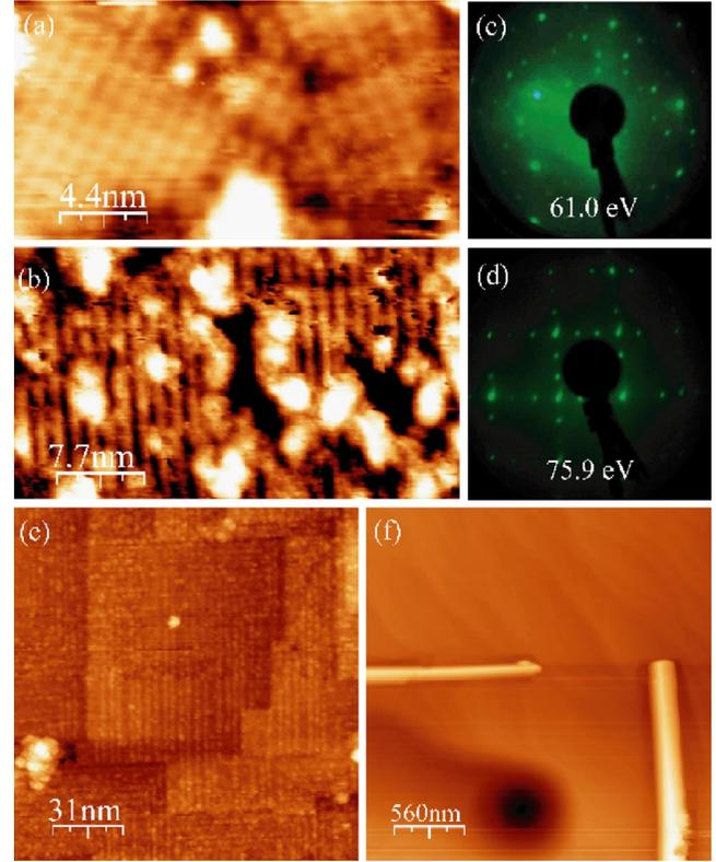
FIG. 1 (color online). STM images of (a)  $(\sqrt{5} \times \sqrt{5})R26.6^\circ$  and (b)  $(3 \times 1)$  reconstructions. LEED patterns of the (c)  $(\sqrt{5} \times \sqrt{5})R26.6^\circ$  and (d)  $(3 \times 1)$   $\text{BaTiO}_3(001)$  surfaces. (e) STM image of nanometer wide stripes on the flat terraces upon annealing above 1373 K. (f) Precipitation on nano-stripe-ordered surface after aggressive annealing for a prolonged time.
