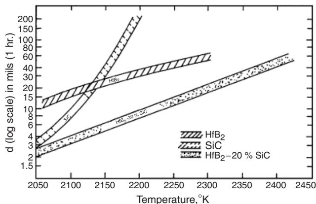
**Fig. 1.** One-hour oxidation resistance of monolithic HfB<sub>2</sub>, monolithic SiC, and HfB<sub>2</sub>+SiC composite (taken from Clougherty, Pober, and Kaufman).<sup>7</sup>
