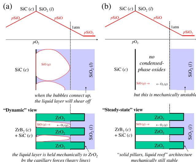
**Fig. 2.** The “dynamic view” (a) and “steady-state view” (b) of why ZrB<sub>2</sub>+SiC has better oxidation resistance than monolithic SiC above the SiO boiling transition temperature.
