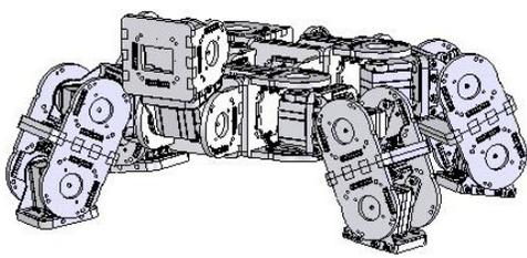
Fig. 1. *Surveyor Dog* 17 modules in a 4-legged configuration
