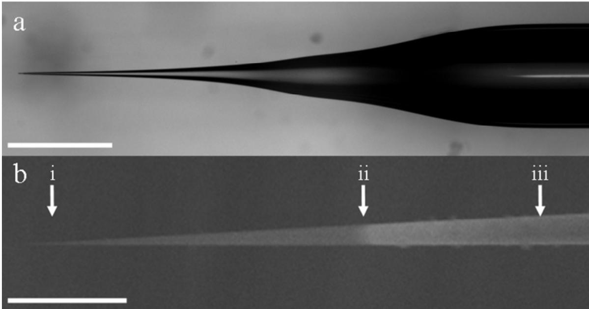
**Figure 1:** CNP for microinjection. (a) Image of a very fine-tipped, blunt taper CNP. Scale bar, 1mm. (b) SEM micrograph (10KV) of the very fine tip of a blunt taper CNP showing the nanoscopic carbon tip (i), the end of the exposed carbon tip (ii), and the quartz micropipette exterior (iii). Scale bar, 10  $\mu\text{m}$ .
