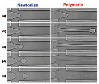
FIG. 2. (Color) Snapshots of drop formation process of both Newtonian (left column) and polymeric (right column) fluids. (Enhanced online.)
