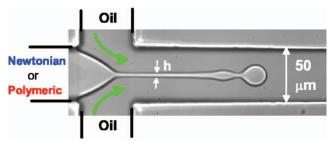
FIG. 1. (Color) Microchannel experimental setup. The device is  $50~\mu m$  wide and  $30~\mu m$  deep. Oil is used as the continuous phase. Newtonian or polymeric fluids are used as dispersed phases.
