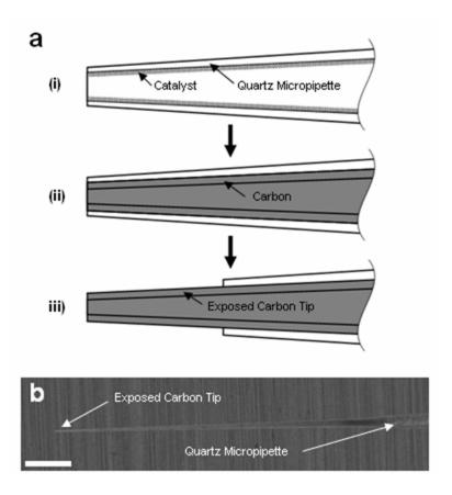
**Figure 1.** (a) CNP fabrication schematic showing (i) internal deposition of catalyst before micropipette pulling, (ii) deposition of carbon by CVD, and (iii) exposing carbon tip by wet-etching. (b) SEM micrograph of a carbon tip integrated into a quartz micropipette. Scale bar, 5 μm.
