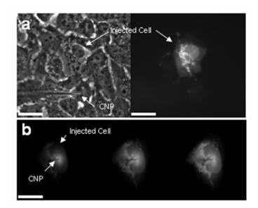
**Figure 5.** (a) Left to right: OSCC before and after fluorescent dye injection with a CNP. Scale bar,  $10 \mu m$ . (b) Left to right: Fluorescent images show an OSCC being injected three times with a CNP. Scale bar,  $10 \mu m$ .
