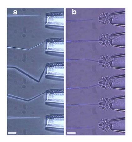
**Figure 3.** (a) From top to bottom: the carbon pipe tip of the CNP buckles when pushed against the wall of a glass pipette and recovers its initial shape once the force is removed. Scale bar, 15  $\mu$ m. (b) From top to bottom: a CNP penetrates through the membrane of an SMC. The cell is held in place by glass micropipette aspiration. Scale bar, 15  $\mu$ m.
