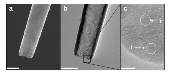
**Figure 2.** (a) SEM micrograph at 15 KV of a CNP tip. Scale bar, 500 nm. (b) TEM micrograph at 200 KV of the same CNP tip. Scale bar, 500 nm. (c) Amorphous (i) and graphitic (ii) carbon is observed with TEM. Scale bar, 10 nm.
