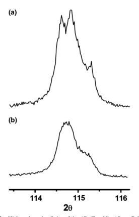
**Fig. 7.** High-angle peak splitting of  $(1-x)Ba(Zn_{1/3}Nb_{2/3})O_3 - xBaNb_{4/5}$   $O_3$  (x = 0.04) after sintering and annealing at 1300°C for 24 h in: (a) a powder of the same composition, (b) ZnO vapor.
