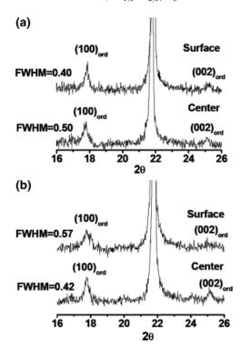
**Fig. 3.** X-ray diffraction patterns of stoichiometric  $Ba(Zn_{1/3}Nb_{2/3})O_3$  sintered (1420°C, 5 h) in its own powder and then: (a) annealed at 1300°C for 24 h in its own powder, (b) re-annealed at 1300°C for 12 h in ZnO powder.
