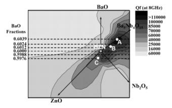
**Fig. 9.**  $Q \times f$  map illustrating the movement of the composition of  $(1-x)Ba(Zn_{1/3}Nb_{2/3})O_3 - xBaNb4/5O3$  (x = 0.04) toward ZnO: (A) starting composition; (B) muffled in ZnO-vapor, (C) muffled in ZnO powder.
