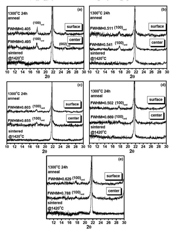
Fig. 1. X-ray diffraction patterns of the surface and interior of stoichiometric  $Ba(Zn_{1/3}Nb_{2/3})O_3$  (BZN) pellets sintered at 1420°C for 5 h and annealed at 1300°C 24 h in muffling environments of: (a) their own powder, (b) sintered in their own powder and annealed in ZnO powder, (c) sintered and annealed in ZnO powder, (d) sintered and annealed in ZnO vapor, and (e) a pellet of BZN+0.5wt%ZnO sintered and annealed in ZnO vapor.
