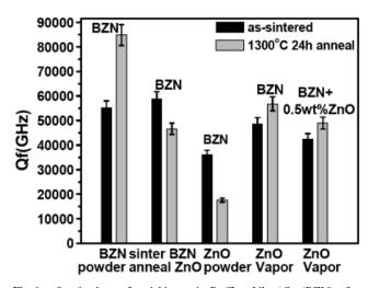
**Fig. 6.**  $Q \times f$  values of stoichiometric Ba(Zn<sub>1/3</sub>Nb<sub>2/3</sub>)O<sub>3</sub> (BZN) after heat treatments in different ZnO-loss-protective environments.
