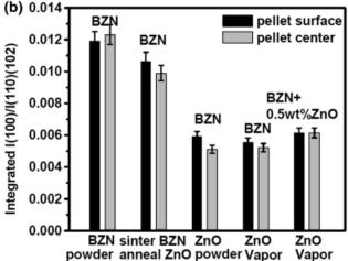
**Fig. 2.** (a) The width (full-width at half-maximum), and (b) the integrated relative intensity of the  $(100)_{ord}$  reflection of  $Ba(Zn_{1/3}Nb_{2/3})O_3$  (BZN) pellets after heating in the different ZnO-loss protective environments shown in Fig. 1. Data are included for the pellet surface and integring
