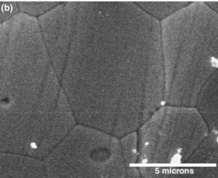
**Fig. 4.** Scanning electron microscope images of a stoichiometric Ba( $Zn_{1/3}$ ) Nb<sub>2/3</sub>)O<sub>3</sub> pellet sintered in (a) its own powder, (b) in ZnO powder.
