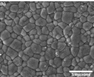
**Fig. 8.** Scanning electron microscope images of the (1-x)Ba( $Zn_{1/3}$ Nb<sub>2/3</sub>)  $O_3-x$ BaNb<sub>4/3</sub> $O_3$  (x=0.04) sintered in (a) its own powder (b) ZnO vapor.
