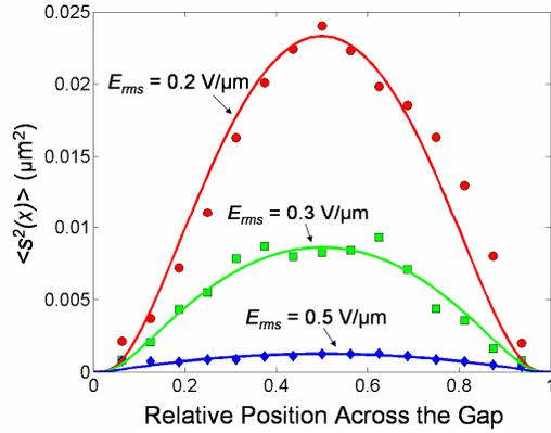
**FIGURE 3:** The variance of the filament's transverse displacement is plotted vs. relative location across the gap at  $E_{rms} = 0.2, 0.3$  and  $0.5 \text{ V}/\mu\text{m}$ . The symbols and lines correspond, respectively, to experimental data and theoretical predictions of a tension-optimized, Brownian dynamics-based model for a clamped rod with flexural rigidity  $\kappa = 7.3 \cdot 10^{-26} \text{ Nm}^2$ .
