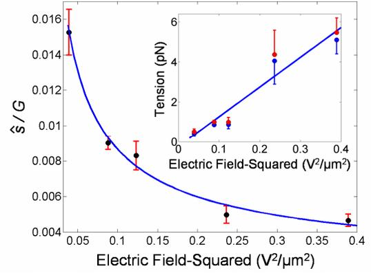
**FIGURE 4:** The average, standard deviation of the displacement ( $\pm 1$  s.e.m.) and the filament's estimated tension obtained from Eq. 2 (+1 s.e.m., red) and from the clamped model (-1 s.e.m., blue) (inset) as functions of the square of the electric field intensity. The solid line is the best fit to the clamped model estimates.
