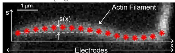
**FIGURE 2:** Contrast-enhanced image of an actin filament trapped across the gap between two electrodes. The image also depicts the discretized position data (\*).
