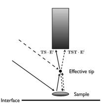
FIG. 2. The simplified model of the collection tip.
