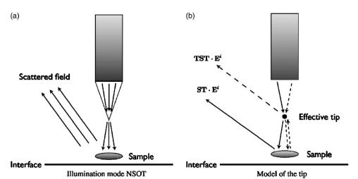
FIG. 1. The simplified model of the illumination tip.
