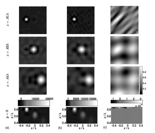
FIG. 5. Comparison of reconstructions from weak tip and strong tip models. The effective tip polarizability is  $\lambda^3/100$ ; column (a) shows the weak tip reconstruction from weak tip simulated data, column (b) is the strong tip reconstruction with strong tip simulated data, and column (c) is the reconstruction with the weak tip model using strong tip simulated data. Images in the first three rows are linearly normalized.
