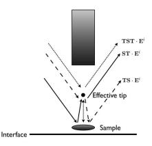
FIG. 3. The simplified model of the apertureless tip.
