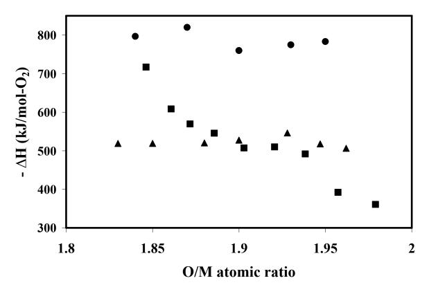
Figure 3. Oxidation enthalpies (- $\Delta H$ ) for ( $\blacksquare$ )  $Ce_{0.8}Ti_{0.2}O_2$ , ( $\blacktriangle$ )  $Ce_{0.81}Zr_{0.19}O_2$  and ( $\bullet$ )  $CeO_2$  as a function of stoichiometry at 973 K.
