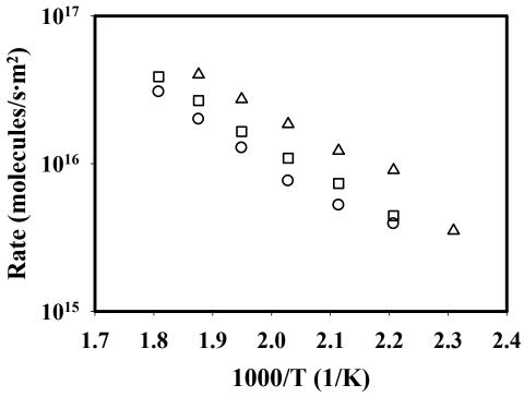
Figure 4. Differential reaction rates for the WGS reaction over ( $\circ$ ) 1wt% Pd/CeO<sub>2</sub>, ( $\square$ ) 1wt% Pd/Ce<sub>0.81</sub>Zr<sub>0.19</sub>, and ( $\Delta$ )1wt% Pd/Ce<sub>0.8</sub>Ti<sub>0.2</sub>O<sub>2</sub>.
