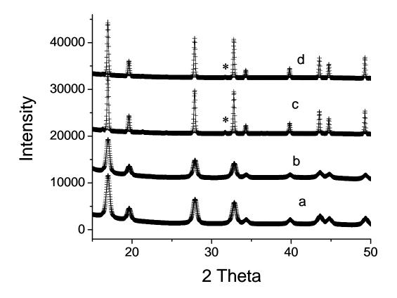
Figure 1. XRD patterns for ceria-titania mixed oxides: a)  $Ce_{0.9}Ti_{0.1}O_2$  calcined at 973 K for 5 h, b)  $Ce_{0.8}Ti_{0.2}O_2$  calcined at 973 K for 5 h, c)  $Ce_{0.9}Ti_{0.1}O_2$  calcined at 1323 K for 5 h, and d)  $Ce_{0.8}Ti_{0.2}O_2$  calcined at 1323 K for 5 h. The calculated profiles are solid lines and the experimental data are marked with + signs. The symbols (\*) show the presence of weak rutile peaks on ceria-titania mixed oxides calcined at 1323 K.
