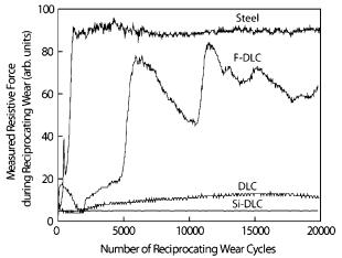
Figure 4. Plot of measured resistive force versus number of reciprocating cycles for wear tests against silicon nitride counter-surface.
