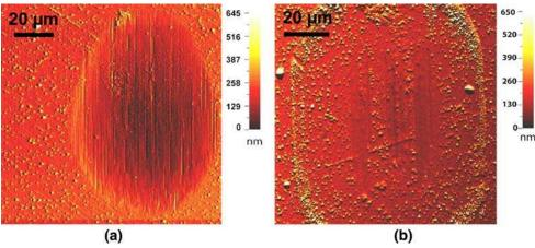
Figure 3. AFM images of wear scars on the Si-DLC films produced by small amplitude reciprocating wear against (a) silicon nitride and (b) PMMA counter-surface.
